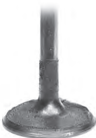
Intake Valve after P.i. Treatment
