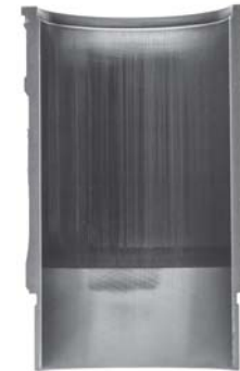
Severely Scuffed Liner
