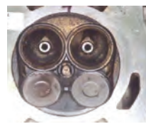
Combustion chamber before P.i. treatment.
