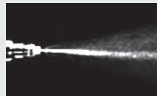
Injector spray pattern before P.i. treatment.
