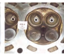
Combustion chamber after P.i. treatment.
