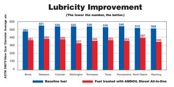
The ASTM D975 diesel fuel standard specifies a wear scar below 520  $\mu$ m in ASTM D6079 testing, while the Engine Manufacturers Association (EMA) specifies a wear scar below 460  $\mu$ m. Testing reveals AMSOIL Diesel All-In-One provides significant lubricity improvement in diesel fuels found across the U.S., delivering improved wear protection.
